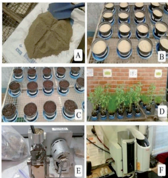
Figure 1. Procedure carried out for gold phytoextraction. Substrate homogenization (A). Substrate disposition (B). Application of vermicomposting (C). Phytoextractor plants (D). Grinder (E). Atomic absorption spectrophotometer (F).
